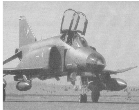
McDonnell F4 phantom aircraft with two General Electric J-79 turbojet engines.
